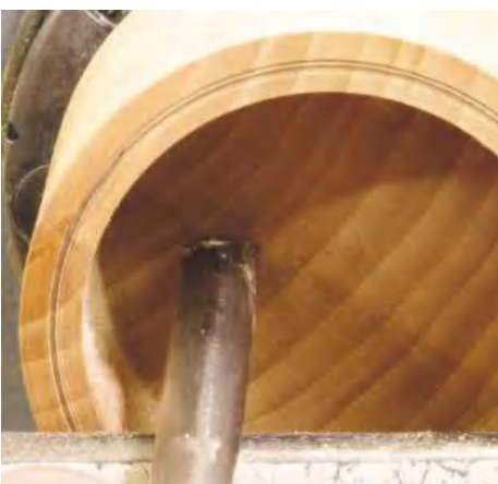
STEP 16. The same tool can be used across the bottom. Keep the tool horizontal and slide it sideways, taking light cuts as you go. Make sure that you don't put the points of the tool in contact with the wood, as it will dig in
